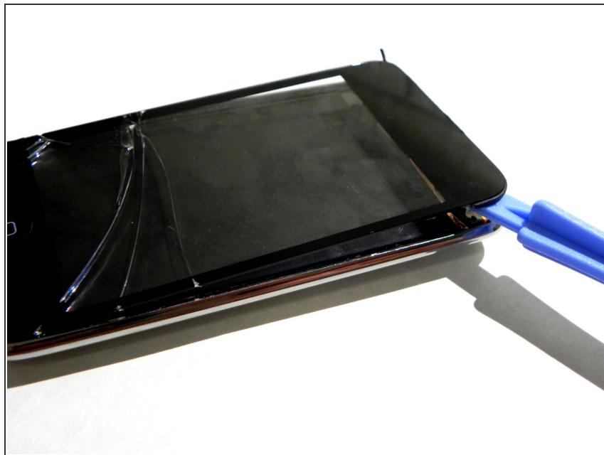
**⚠** Make sure not to slide the tool along the edge once you've managed to wedge it between the screen and panel. Repeat the process of prying the tool into a point along one of the edges and remove the tool to insert it at another point.
